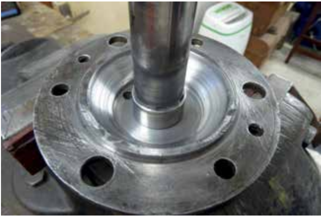
Fig 3. Modified hub with sleeve fitted
